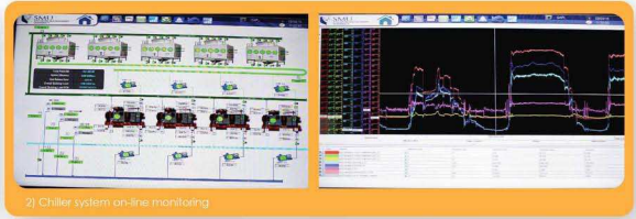
2) Chiller system on-line monitoring
